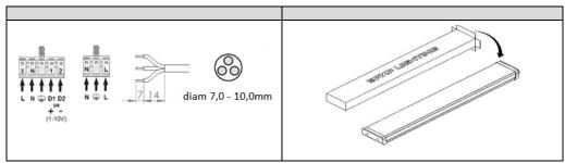
Light source used in this luminaire should be changed by the producer or its service representative or similarly qualified person. Installation kit supplied with the luminaire does not include anchors for wall installation.
